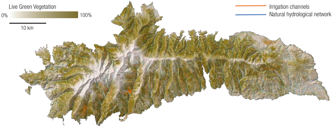
Distribution of the natural hydrological network in Sierra Nevada (blue) in comparison with the network of ancient irrigation channels (orange). The background image shows photosynthetically active vegetation (green), bare soil and snow (both light coloured).USGS/NASA Landsat 5 TM 2011-06-19. Irrigation channel data courtesy of EU F7 MEMOLA project.
